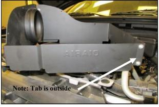
4. Assemble the two Quick Fit panels (#3 & #4) as shown using four 6-32 screws (#9) flat washers (#11) and kep nuts (#10).
