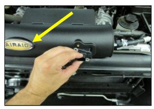
8. Apply the Airaid Decal as shown. Transfer the MAF sensor into the Airaid Intake Tube (#2) and secure using two 8-32 x 1/2" button head screws (#11). **Do Not Use The Factory Torx Head Screws!**
