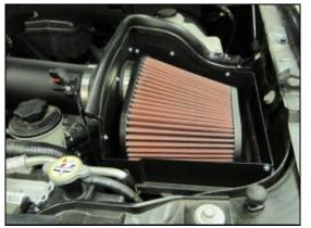
**10.** Install the Airaid Premium Filter (#1) to the mounting flange inside the quick fit assembly. Complete the installation by attaching the Weather Strip (#5) to the top of the panels as shown.
