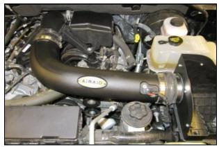
9. A.) Insert the Airaid Intake Tube into the couplers as shown. Check for alignment, and tighten all
