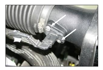
7. Reinstall the **MAF** sensor into the Airaid Adapter Tube using two 8-32 x 3/8" button head screws (#11). **Do Not Use The Factory Screws!**
