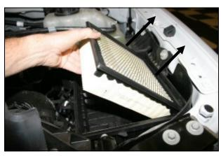
**3.** Remove the factory air filter from the airbox base.
