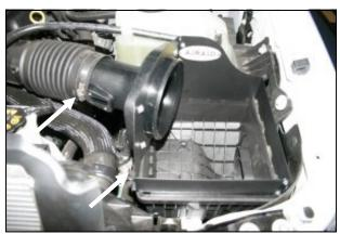
**6.** Install the Quick Fit Assembly onto the top of the factory airbox base sliding the four tabs on the panel into the slots on the base and then latching the three factory latches. Slide the factory intake tube over the **MAF** tube and tighten the factory hose clamp as
