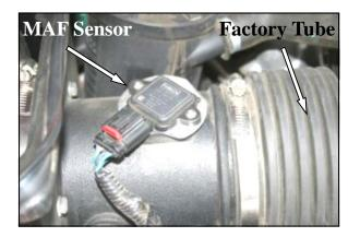
**10.** Install the **MAF** sensor into the Calibration Plate on the Cool Air Box using two 8-3/8" button head bolts (#9), as shown. Reconnect the **MAF** sensor wiring harness.
