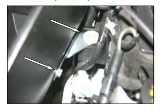
**8.** Reinstall the factory bolt that was removed in step #3, through the bracket that is bolted onto the side of the Cool Air Box. Adjust the box for fit, and tighten both bolts.
