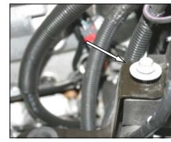
**3.** Remove one bolt from the factory airbox mounting plate, and save it for reinstallation in step #8.
