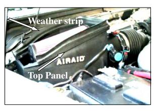
11. Install the Airaid Premium Filter (#1) onto the filter adapter, and tighten the hose clamp. Next install the Top Panel (#3) onto the top of the Cool Air Box using six 8-32x3/8" button head bolts (#9), and #8 flat washers (#10). Install the weather strip (#5) onto the edge of the top panel as shown
