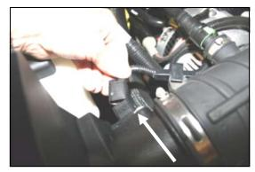
**12.** Reconnect the wiring harness to the **MAF** sensor.
