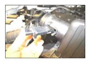
**6.** Using the supplied #20 Torx bit, remove two screws, and remove the Mass Air Flow sensor from the factory air cleaner lid. Save the MAF sensor for later use in step #9.
