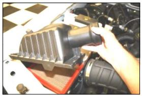
**4.** Slide the factory intake tube off of the factory air cleaner lid, and remove the lid from the vehi-
