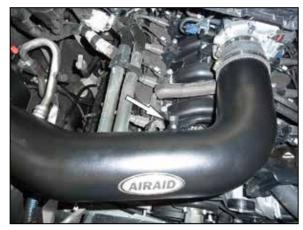
22. Install the longer vent hose assembly onto the AIRAID intake tube and then into the factory vent line as shown.
