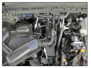
2. Release the spring clamp that secures the EVAP vent line to the intake plenum. Then release the locking tap on the Crankcase vent fitting and disconnect the crank case vent from the intake plenum. 3. Disconnect the vent line from the intake plenum where shown, then unhook the heater hose clip from the intake plenum.
