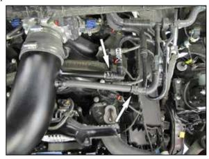
21. Install the shorter vent hose assembly onto the AIRAID intake tube and then connect the other end into the EVAP vent line.
