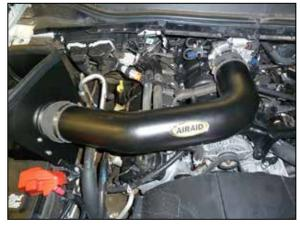
19. Install the AIRAID intake tube into the hump coupler and then into the step coupler at the throttle body, adjust the tube for best fit and then secure with the provided hose clamps.
