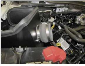
15. Install the provided hump coupler (08418) onto the filter adapter and secure with the provided hose clamp.
