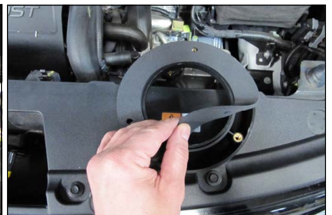
6. Prepare the Filter Adapter for installation by positioning the Adapter Gasket on the mounting side and lining up the holes.
