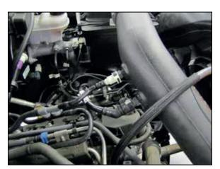
9. Connect the EVAP and crank case vent lines to the quick connect fittings installed into the AIRAID<sup>®</sup> intake tube.
