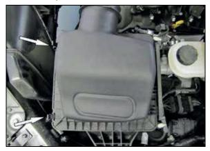
4. Release the two clips that secure the upper air filter housing and then remove the upper housing and factory air filter.
