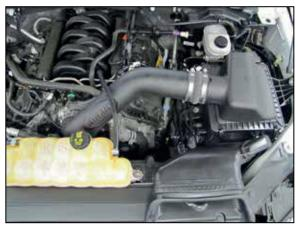
10. Double check your work!Make sure there is no foreign material in the intake path.Make sure all clamps, hoses, bolts, and screws are tight.Double check the hood clearance!Reconnect the negative battery cable!
