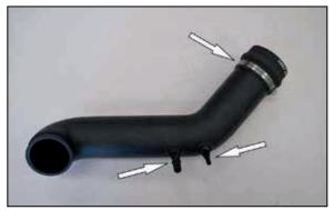
6. Install the provided vent fittings into the AIRAID<sup>®</sup> intake tube as shown. Install the provided hump coupler (08683) onto the intake tube and secure with the provided hose clamp.
