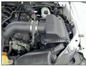
8. Install the AIRAID<sup>®</sup> intake tube into the coupler at the air filter housing and then into the coupler at the throttle body, adjust the tube for best fit and then secure with the provided hose clamps.
