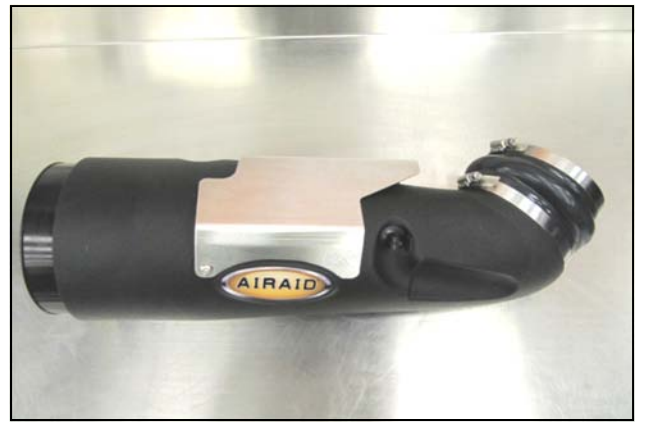
12. Slide the Hump Hose and Clamps onto the Airaid Intake Tube. Leave the clamps loose for now.
