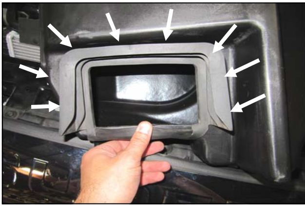
10. Transfer the factory airbox coupler from the OEM airbox inlet into the Airaid Cold Air Box, or C.A.B.
