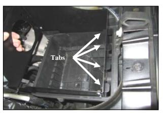
**5.** Install the assembly onto the lower half of the factory airbox. Slide the metal tabs into the airbox slots, and fasten the 3 airbox clips.
