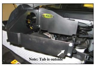
**4.** Assemble the two Quick Fit panels (#3 & #4) as shown using four 6-32 screws (#7) flat washers (#9) and kep nuts (#8). Apply the Airaid Foil Decal onto the Panel as shown.
