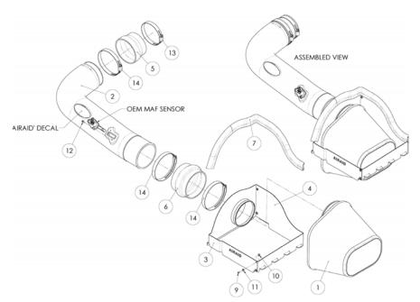
1. Disconnect the negative battery cable! Loosen the two intake clamps, unclip the coolant hose and remove the Factory intake tube.
