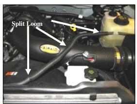
9. A.) Insert the Airaid Intake Tube into the couplers as shown. Check for alignment, and tighten all
