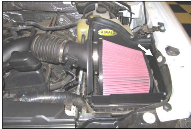
14. Install the Airaid Premium Filter on to the Air Meter Tube and tighten the clamp.
