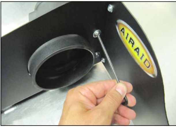
10. Install the Air Meter Tube into the Panel Assembly and secure using the two 1/4-20 Button Head Screws ,and 1/4" Flat Washers .
