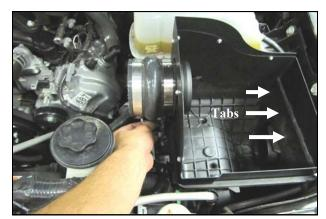
6. A.) Install the Silicone Hump Hose (#7) and two #64 Hose Clamps(#14) onto the Quick Fit assembly
