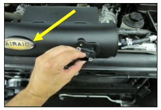
8. Apply the Airaid Decal as shown. Transfer the MAF sensor into the Airaid Intake Tube (#2) and secure using two 8-32 x 1/2" button head screws (#11). Do Not **Use The Factory Torx Head Screws !**
