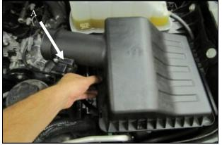
2. A.) Disconnect the Mass Air Flow (MAF) Sensor.
