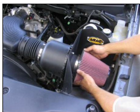
11. Mount the Airaid air filter on to the filter adapter using the supplied hose clamp.
