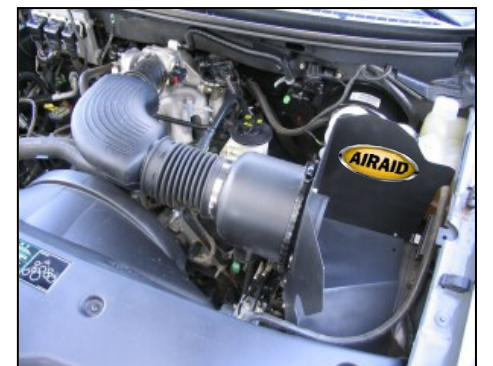
8. Install the Airaid Cool Air Dam assembly on vehicle using the factory intake tube clamp. Apply the Airaid Foil Decal onto the Panel as shown.
