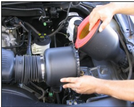
1. Disconnect negative battery cable. Unclip factory filter housing from intake assembly.
