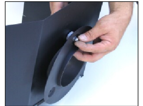
4. Assemble the Airaid Filter Adapter plate using the supplied 1/4 inch bolts, washers, spacers and nuts provided as shown above.
