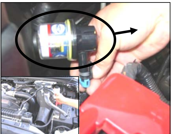
4. Disconnect the electronic filter restriction gauge wiring harness, remove the restriction gauge, and the rubber grommet. (Note: retain these parts for reuse.) Remove the air filter inlet tube and hose assembly (see inset picture). USE CAUTION when removing these elements, as it is a tight fit. Be careful not to tear the factory insulation around the radiator support.
