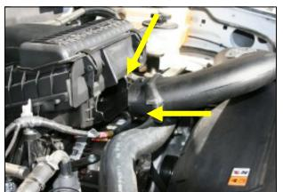
**5.** Install the top of the Airaid MIT into the stock airbox pushing down and in. (*It will snap into place.*)
