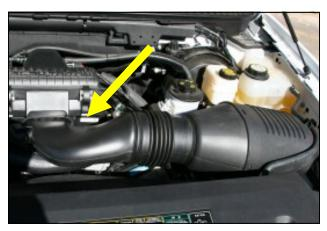
**1.Disconnect The Negative Battery Terminal!** Disconnect intake tube from air filter housing by unsnapping the tube assembly from the housing.
