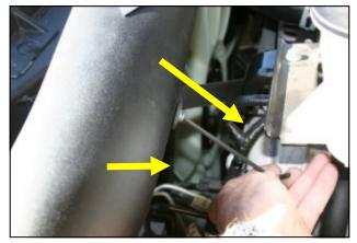
7. Install the 1/4"x 20 Allen bolt and washer thru the bracket and into the MIT . Make your final adjustments and tighten the Allen bolt, and the nut on the power steering bracket. The MIT should not make contact with the radiator support or inner fender.
