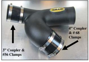
**5.** Slide the Couplers and Clamps onto the Intake tube as shown. Apply the Airaid Bubble Decal onto the Intake Tube as shown.
