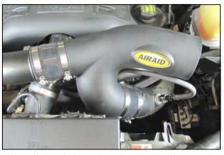
**6.** Install the Airaid Intake Tube onto the factory turbo plumbing and tighten the Clamps. Reconnect the vacuum line if so equipped
