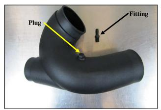
**4.** On late model vehicles, Install the 1/4" Plug into the Airaid Intake Tube as shown.
