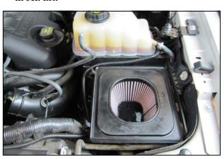
**3.** If installing an Airaid Jr. kit, replace the factory air filter with the Airaid Premium Filter at this time.
