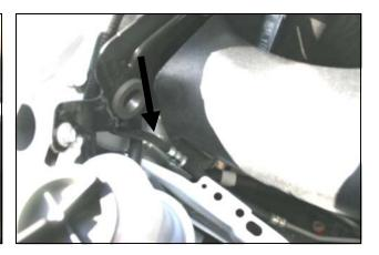
**9.** Due to inconsistent factory tolerances, some minor adjustment may be necessary to the factory A/C line so it will clear the Airaid MIT near the radiator support.. When all adjustments have been completed, tighten the nut, and button head bolt at the L-bracket.
