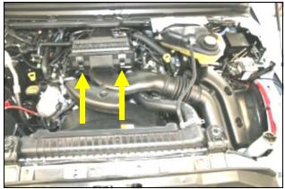
**2.** Grab the factory intake tube just above the fan shroud, and with a sharp lifting motion, remove it from the air cleaner housing.
