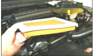
**4.** Unclip the two latches that hold the air cleaner tray into the air cleaner.
