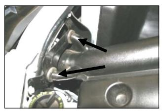
**3.** Remove the factory tube from the radiator support by pulling the tube out of the grommets. There are no bolts holding the tube. Remove the factory tube from the vehicle.
