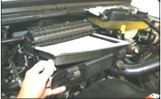
**6.** Install the Airaid Premium Filter (#1) into the factory airbox tray, slide it back in, and relatch the two clips.
