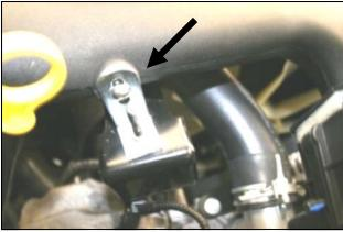
**8.** Install the L-bracket (#3) over the factory stud re-using the nut removed in step #1. Next install the button head bolt (#4) and washer (#5) thru the L-bracket, and into the tube. Leave loose until final adjustments have been made.
