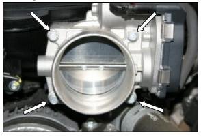
2. Remove the four bolts from the throttle body, and remove the throttle body from the intake manifold, and set it aside. There's no need to disconnect the wiring harness.
