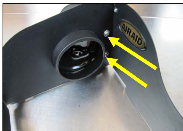
11. Mount the Sensor Tube onto the Panel Assembly and secure using the two 1/4-20 Button Head Screws and 1/4" Flat Washers.
