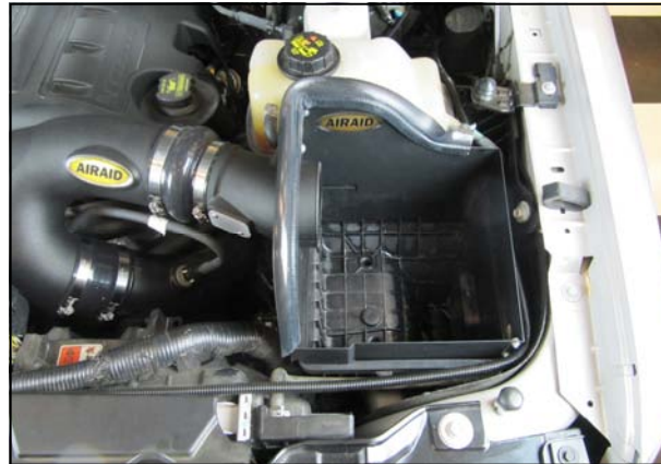
14. Tighten the Clamps on the Hump Hose, reconnect the MAF or MAP sensor and install the Weather Strip as shown, with the contour rolling away from the Filter area.
