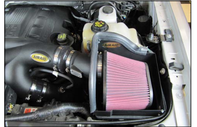
15. Install the Airaid Premium Filter onto the Sensor Tube and tighten the clamp.
