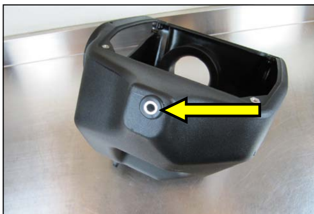
7. Insert the 5/8" Grommet and Spacer into the opposite side of the Airaid Air Box.
