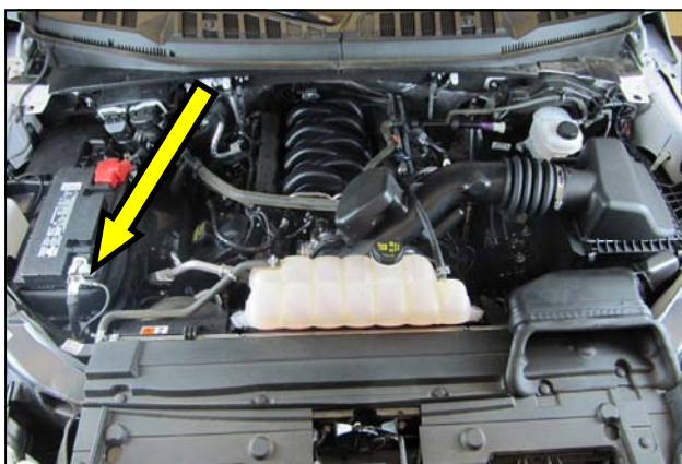
1. Disconnect the negative battery terminal.
