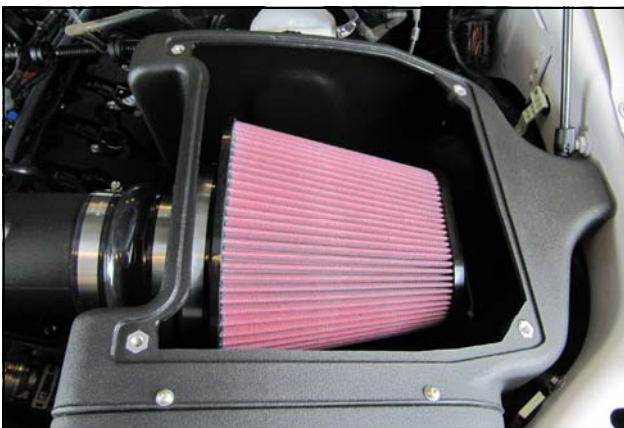
19. Install the Airaid Premium Filter onto the Filter Adapter and tighten the clamp.
