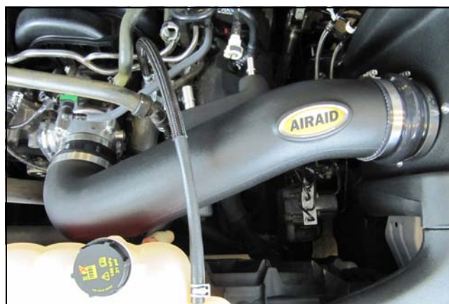
17. Insert the Airaid Intake Tube into the throttle body coupler, then into the Air box Hump Hose. Rotate the Tube forwards and backwards until proper alignment is achieved and tighten all four Clamps. Apply the Airaid Decal onto the Tube as shown.
