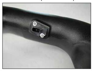
11. Remove the mass air sensor from the factory air filter housing and install it into the AIRAID® intake tube using the provided hardware and spacers. Install the AIRAID® decal onto the intake tube.
