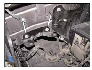
5. Remove the two bolts that secure the air filter housing mounting bracket to the inner fender and remove the bracket from the vehicle.
