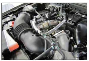
3. Loosen the hose clamp that secures the factory intake tube to the turbo inlet, release the four clips that secure the upper air filter housing and then remove the assembly from the vehicle.
