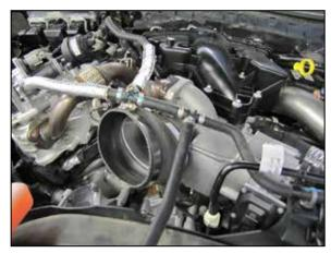
10. Install the provided coupler (08695) onto the turbo inlet and secure with the provided hose clamp.
