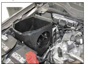
9. Install the AIRAID® housing into the vehicle so the mounting stud inserts into the mounting grommet and the fresh air intake opening sits around the fresh air duct. NOTE: Be sure not to pinch the wiring harness between the fresh air duct and AIRAID® housing.
