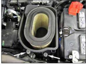
4. Remove the two bolts that secure the lower air filter housing to the mounting bracket, then pull the lower air filter housing straight up to dislodge it from the mounting grommets and remove it from the vehicle.
