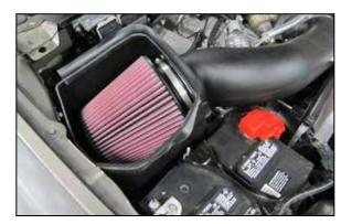
13. Install the air filter onto the intake tube and secure with the provided hose clamp.
