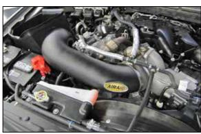
12. Install the AIRAID® intake tube into the AIRAID® housing and into the coupler at the turbo inlet. Adjust the tube for best fit and then secure with the provided hardware and hose clamp.
