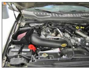
**16. Double check your work!**Make sure there is no foreign material in the intake path. Make sure all clamps, hoses, bolts, and screws are tight. Double check the hood clearance!
