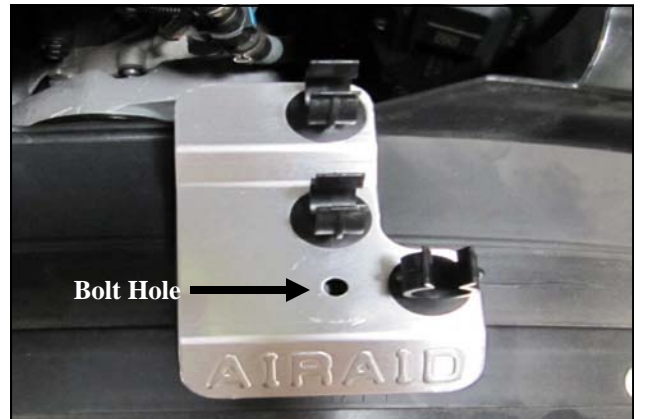
15. Insert the three remaining Hose Anchors into the Hose Bracket as shown.
