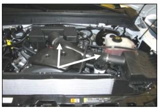
**1. Disconnect the negative battery cable!** Loosen the two intake clamps, unclip the coolant line, and remove the Factory intake tube.
