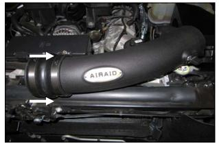
**7.** Install the Hump Hose (#5), and the clamps (#13) onto the Intake Tube. Slide the hump hose and clamps down the tube as far as they will go and leave the clamps loose for now. Apply the Airaid Bubble Decal inside the Airbox as shown.
