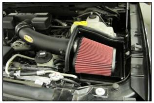
**10.** Install the Airaid Premium Filter (#1) to the mounting flange inside the quick fit assembly. For **SVT Raptor** vehicles:
