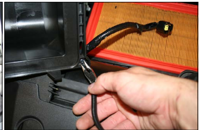
3. Using a pair of needle nose pliers, carefully compress the fins of the wiring harness anchor and pull it out of the air box lid.
