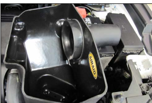
7. Install the Filter Adapter to the inside of the Cool Air Box, using the three 1/4"-20 hex head bolts and 1/4" flat washers. Apply the Airaid Bubble Decal inside the Air-box as shown.
