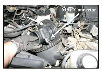
4.Unlatch the clamp on the canister to separate the two halves. Once separated, remove the factory air filter. A) Next, slide the large round plastic Mass Air Flow (MAF) sensor adapter plate from the canister. To do this, slide the wires thru the rubber grommet to gain access to the MAF sensor wiring connector. Now disconnect the MAF sensor wiring harness, and remove the MAF sensor housing and adapter plate. Remove the remaining half of the canister from the vehicle.
