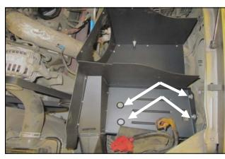
**8.** Place the **CAD** assembly in the engine compartment and start the four factory bolts from step 4. Leave the bolts loose for now.
