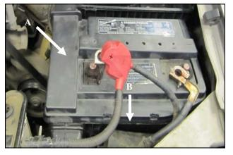
**3. A.)** Remove the factory battery cover. **B.**) Using a 5/16" socket, remove the factory battery hold down.
