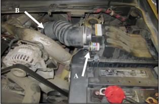
2. A.) Disconnect the filter minder in the top of the airbox.
