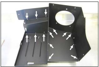
5. Create the Cool Air Dam, or CAD assembly as shown using the Bottom Panel (#3), Side Panel (#4), and the 8-32 Thread Cutting Screws (#17). NOTE: Panel tabs are to be on the bottom of its mating panel.
