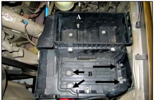
4. A.) Disconnect the air temp sensor. **B.**) Remove the four bolts securing the air/battery box assembly to the vehicle. Remove the assembly and set aside. The bolts and air inlet will be reused.
