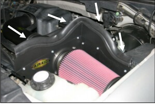
12. If your vehicle Does Not have a hood mat, install the panel extension (#4) as shown using five 6-32 Phillips head screws (#5), flat washers (#6), and keps nuts (#7). Next install the weatherstrip (#4) onto the top of the panel assembly as shown.
