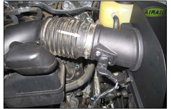
12. Slide the factory intake tube onto the Airaid Tube and tighten the clamp. Reconnect the Mass Air Flow or MAP sensor.
