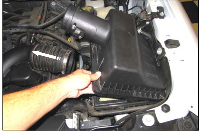
3. Slide the factory intake away from the airbox. Lift up and slide the airbox tabs out of the slots in the lower half and set aside.
