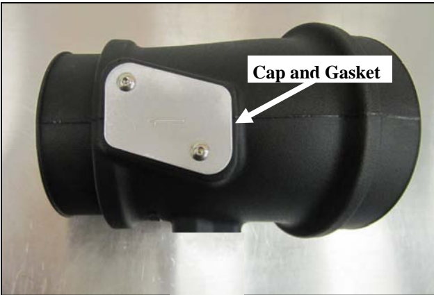
7. If your vehicles intake utilizes a MAP sensor: Install the Meter Cap and Gasket onto the Airaid Intake tube as shown, using the two 8-32 1/2" Button Head Screws.
