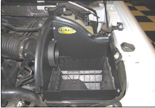
13. Install the Weather Strip to the Panel assembly as shown, with the contour rolling away from the filter area.
