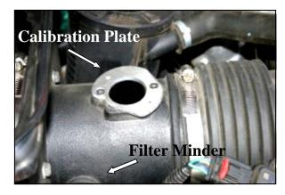
**9.** *A.*) Install the Calibration Plate onto the Cool Air Box using two 8-32 x 1/2" Flat Head Screws (#14). *B.*) Reinstall the factory grommet, and filter minder into the Cool Air Box, and then reconnect the filter minder wiring harness.
