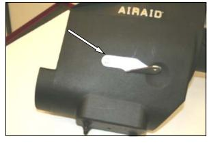
**5.** Install the bracket (#11) using one 1/4-20x5/8" hex bolt (#6), 1/4" flat washer (#7), and 1/4-20 serrated nut (#8) as shown. Just snug the bolt for now, it will need to be adjusted in step #8.
