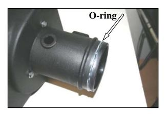
**6.** Install the O-ring (#17) into the groove on the Cool Air Box as shown. Apply a *light* coat of the supplied grease onto the O-ring.
