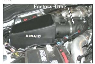
**7.** Apply a *light* coat of the supplied grease onto the inside of the factory tube. Install the Airaid Cool Air Box into the vehicle making sure it is seated correctly into the factory grommets, and the inlet is aligned with the factory hole in the fender. Slide the factory intake tube over the O-ring and then tighten the factory hose clamp.
