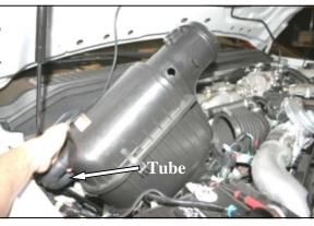
**2.** Remove the factory airbox and tube from the vehicle as an assembly, by pulling straight up on the box. It is only held in place by grommets, no bolts.
