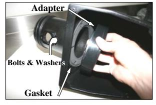
**4.** Install the adapter gasket (#12), and filter adapter (#4) into the Airaid Cool Air Box (#2) using three 1/4-20x5/8" hex bolts (#6), and 1/4" flat washers (#7).
