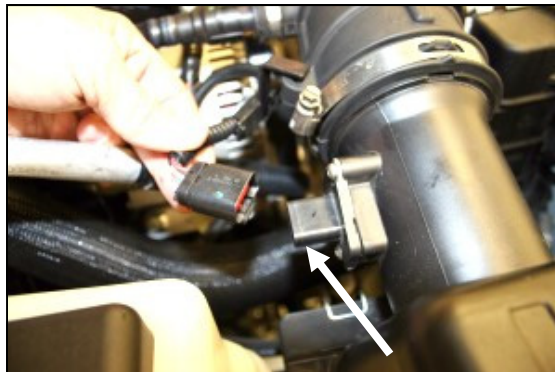
2. Slide the red tab on the bottom of the Mass Air Flow sensor wiring connector and then squeeze the connector, and unplug the harness from the sensor.
