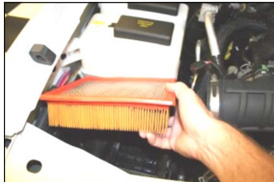
5. Remove the factory air filter from the factory air cleaner base.
