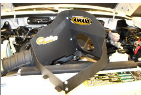
7. Assemble the two Quick Fit Panels (#2&3), using five 6-32 screws (#9), #6 flat washers (#10), and nuts (#11). Apply the Airaid Foil Decal onto the Panel as shown.
