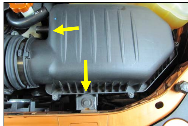
3. Separate the crankcase breather from the air box lid and remove the air box screw in the core support. Lift the air box / tube assembly out of the vehicle and set the screw aside, it will be reused in step 6.
