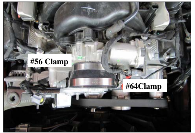
12. Slide the Reducing Coupler and the # 56 and 64 Clamps onto the throttle body. Leave the Clamps loose for now.
