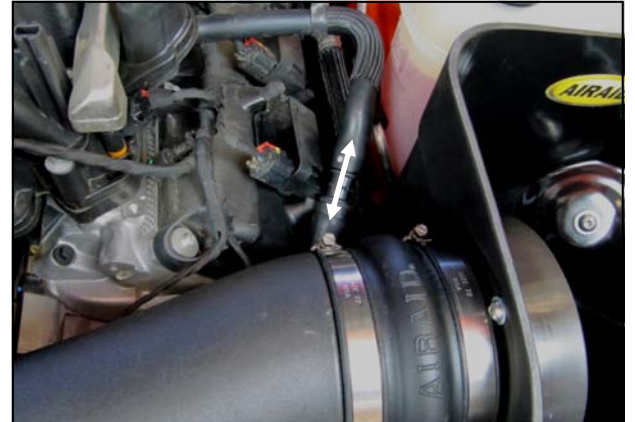
15. Connect the Barbed Fitting in the PCV hose to crank case breather line in the valve cover .
