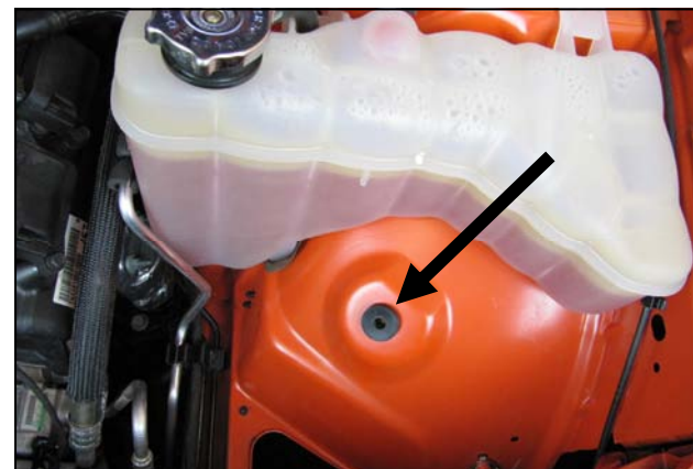
6. Set the Well Nut into the hole in the inner fender.
