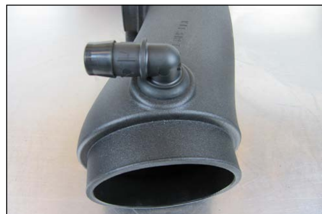
9. Insert the 3/4" Grommet and Barbed Elbow into the Airaid Intake Tube as shown.
