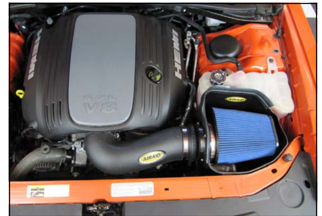
18. Reinstall the engine cover and oil cap. Reconnect the negative terminal on the battery.
