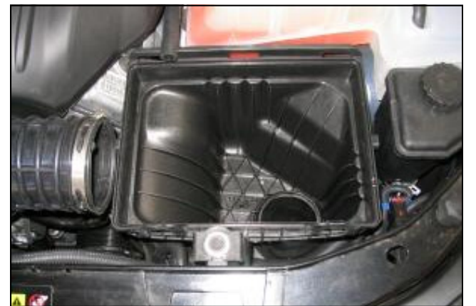
3. Remove the factory air box lid and flat panel filter. ( Note: Retain the factory air box base. )
