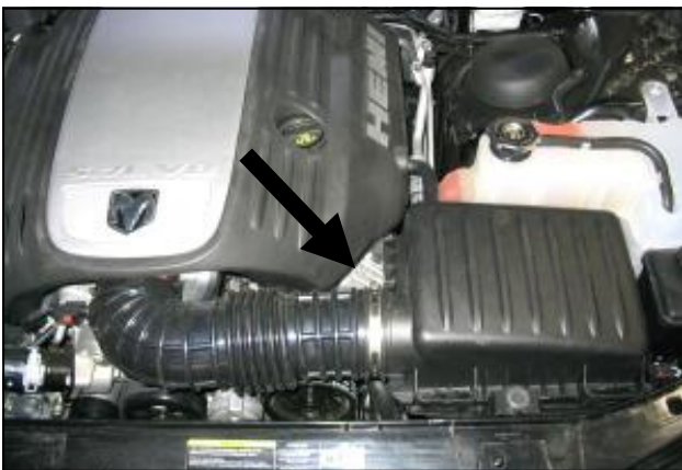
1. Loosen the hose clamp on the intake tube.
