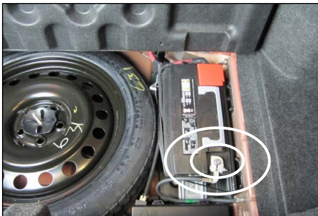
1. Disconnect the negative battery terminal, located in the trunk, by the spare tire.
