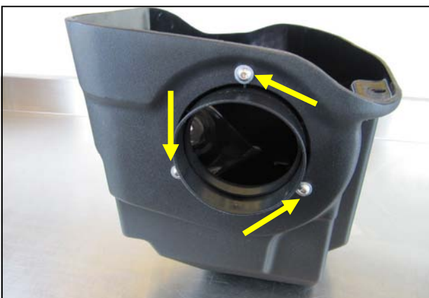
5. Install the Filter Adapter onto the Cool Air Box using the three 1/4" Button Head Screws and 1/4" Flat Washers.
