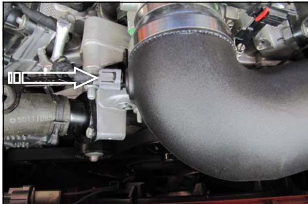
14. Reconnect the air temperature sensor.
