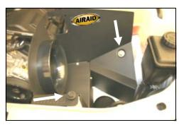
**10.** Install the **CAD** into the vehicle. Reinstall the factory bolt removed in step #6 thru the **CAD** and into the radiator support. Next install the 3/8-16 x 1 1/4" button head bolt (#11) and 3/8" flat washer (#12) thru the **CAD** and into the well nut. Tighten both bolts.
