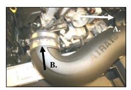
**13. A.** Install the urethane hump hose (#7) onto the filter adapter using two #72 hose clamps (#20), (*Leave loose for now*). **B.** Install the large end of the reducing coupler (#8) on the Airaid Intake Tube (#4), using two #52 hose clamps (#19). Tighten *only* the hose clamp on the tube.
