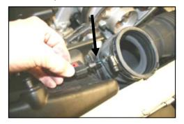
**4.** Lift the intake tube towards you, and without disconnecting the wiring harness, gently remove the temperature sensor from the factory intake tube, and set it aside.
