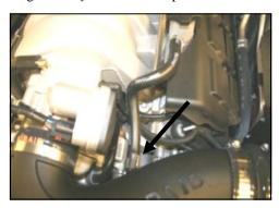
**16.** *If you are working on a 5.7L, skip to step #17.* If you are working on a 6.1L, reconnect the factory breather tube to the Airaid Intake Tube as shown.
