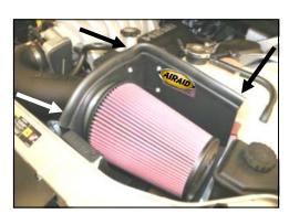
**18.** Install the Airaid Premium Filter (#1), onto the filter adapter inside of the **CAD**, and tighten the hose clamp. Next install the weather strip (#10) onto the top of the **CAD**.
