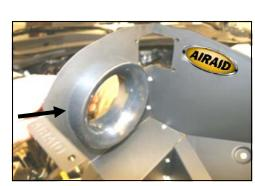
**8.** Next, install the filter adapter (#5) using three  $\frac{1}{4}$  - 20 x  $\frac{1}{2}$ " button head bolts (#13), and  $\frac{1}{4}$  flat washers (#14).
