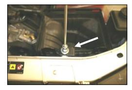
**6.** With a 10mm socket, remove and save the bolt that holds the factory air filter base to the radiator support. Remove the air filter base from the vehicle.
