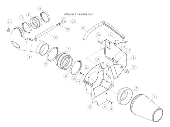
**1.** Disconnect the negative battery cable. If you are working on a 5.7L, first remove the engine beauty cover by lifting it up off of the grommets. Next, loosen the hose clamp that holds the factory intake tube to the throttle body.
