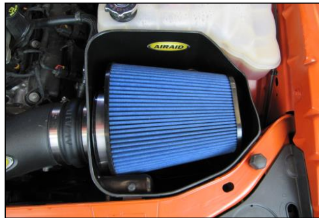
16. Install the Airaid Premium Filter onto the Filter Adapter.
