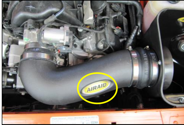
13. Insert the Intake Tube assembly into the Hump Hose first, then into the Coupler onto the throttle body. Tighten all four Clamps at this time. Apply the second Airaid Decal onto the Intake tube.
