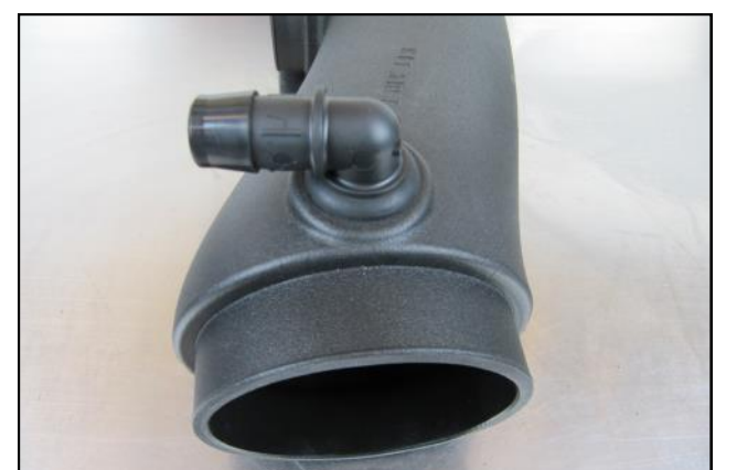
9. Insert the 3/4" Grommet and Barbed Elbow into the Airaid Intake Tube as shown.
