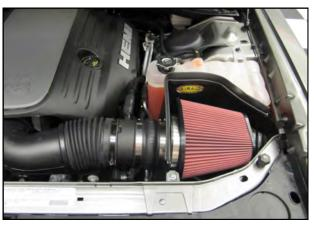
17. Install the Weatherstrip onto the top edge of the Panels with the contour rolling away from the Filter area. Complete the installation by attaching the Airaid Premium Filter to the Filter Adapter.
