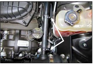
**16.** For **3.6L V6 Pentastar equipped vehicles:** Install the Smaller, 5/8" hose onto the Barbed Fitting and factory hard line. Snap a Speed Clamp on each end of the hose to secure it in place.
