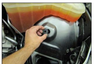
7. Place the 3/8 " Well Nut into the hole in the inner fender. It will be fully secured later in step 9.
