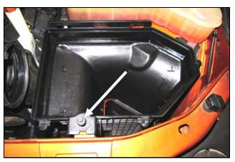
**2.** Remove the core support bolt securing the lower half of the airbox and remove it from the vehicle.
