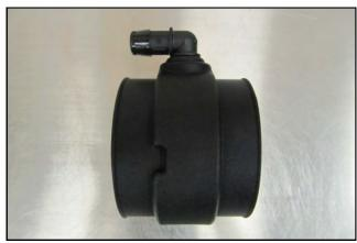
13. For 6.4L V8 SRT-8 equipped vehicles: Locate the V8 Airaid Intake Tube marked KIT-210-8T and insert the larger, 3/4" Grommet into the side. Complete the SRT-8 Tube assembly by inserting the 5/8" 90 Degree, Barbed Fitting into the Grommet as shown.
