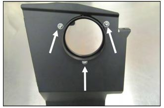
**5.** Install the Filter Adapter onto the Front Panel as shown using three 1/4-20 Button Head Screws and 1/4" Flat Washers.
