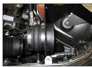
**14.** Install the Hump Hose and Clamps onto the Filter Adapter. Leave the Clamps loose for now.
