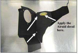
**4.** Create the panel assembly. Join the Front and Rear panels together using the two #6-32 Screws, #6 Flat Washers, and #6 Kep Screws. Note: The Tab on the Front Panel is to be behind the Rear panel when properly installed.
