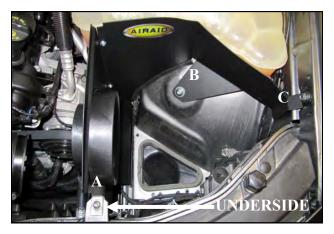
**9.** Lower the Panel Assembly into the inner fender area and align the mounting holes. Be sure to insert the bottom of Front Panel between the ABS line and the sheet metal. Secure the assembly using:
