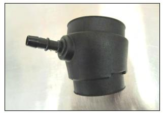
11. For 3.6L V6 Pentastar equipped vehicles: Locate the V6 Airaid Intake Tube marked KIT-210-6T and insert the smaller, 5/8" Grommet into the side. Complete the V6 Tube assembly by inserting the smaller, 5/8" Barbed fitting into the Grommet.
