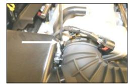
1. Disconnect the negative battery cable. Loosen the hose clamp that holds the factory intake tube to the throttle body.
