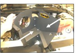
7. Assemble the Airaid Cool Air Dam (**CAD**) panels (#2, #3) using five 6-32 x 5/16" screws (#16), #6 flat washers (#17), and 6-32 keps nuts (#18). Apply the Airaid Foil Decal onto the Panel as shown.
