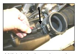
4. Lift the intake tube towards you, and without disconnecting the wiring harness, gently remove the temperature sensor from the factory intake tube, and set it aside.
