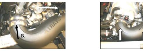
**14.** Install the Airaid Intake Tube into the hump hose first, and then onto the throttle body, making sure it is flush against the throttle body, adjust for fit, now tighten all of the hose clamps.
