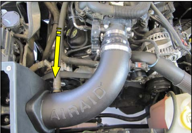
15. Reconnect the factory crank case breather line to the Airaid Intake Tube.
