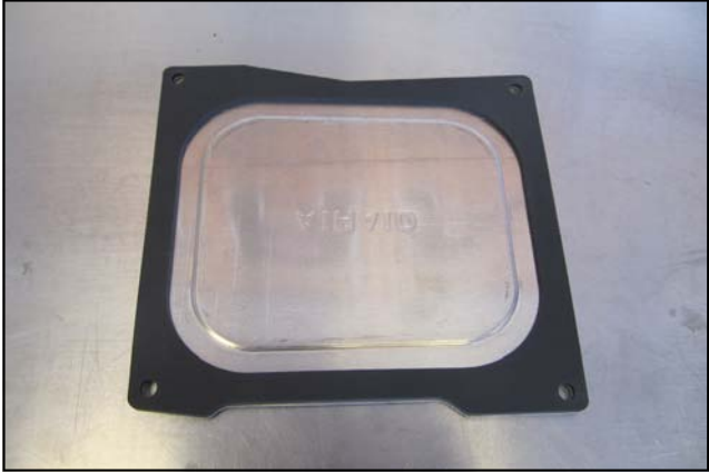
17. Mount the self adhesive Gasket (#7) onto the underside of the Air Box Lid (#6) and peel off the protective film on the top. Mount the lid onto the Air Box using four remaining 1/4-20 x 1/2" Button Head Bolts (#10), and 1/4" Flat washers (#12).
