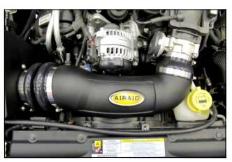
14. Install the Airaid Intake Tube onto the Cold Air Box and throttle body, align, and tighten all four of the Clamps. Reconnect the air temp sensor.
