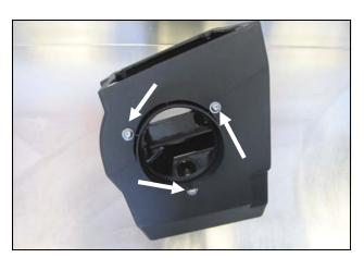
**4.** Install The Filter Adapter in the Cold Air Box using three 1/4-20 x 1/2" Button Head Bolts and 1/4" Flat Washers.
