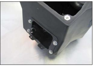
**5.** Install the Air Scoop Bracket onto the Cold Air Box as shown by using four  $1/4-20 \times 5/8$  Hex Bolts , 1/4" Flat Washers, and 1/4" Nylock Nuts.
