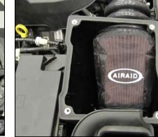
21. Pre Filter Option: Part Number 799-445 For maximum protection in the harshest environments Airaid offers a slip on Pre Filter.
