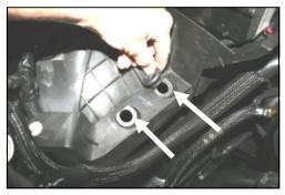
6. Remove the 2 lower grommets from the factory plastic air cleaner mount.
