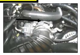
2. Loosen the intake tube hose clamp on the throttle body.
