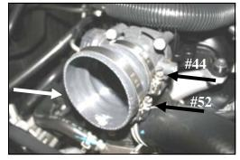
**15.** Install the reducing hump hose (#5) onto the throttle body as shown, with the #44 hose clamp (#15) on the back, and the #52 hose clamp (#16) on the front. Leave the clamps loose for now.
