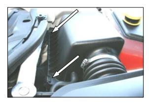
**2.** Unlatch the two clips on the front of the factory airbox lid.
