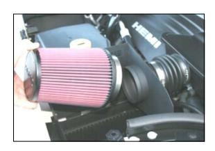
**8.** <u>Install the Airaid Premium Filter</u> (#1) onto the tube on the Quick Fit Panels, and tighten the clamp.
