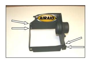
**5.** Assemble the Quick Fit Panels (#2, #3) using four 6-32 x 5/16" screws (#5), #6 flat washers (#6), and 6-32 keps nuts (#7). Apply the Airaid Foil Decal onto the Panel as shown.
