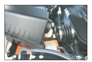
**3.** Remove the factory airbox lid by sliding it forward, and then up and out of the factory intake tube.
