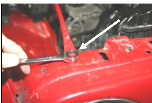
10. Remove and save the bolt from the passenger side radiator support brace. It will be re-used in step #13.
