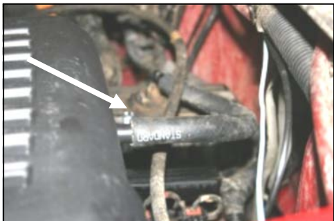
4. Disconnect the breather hose from the resonator.
