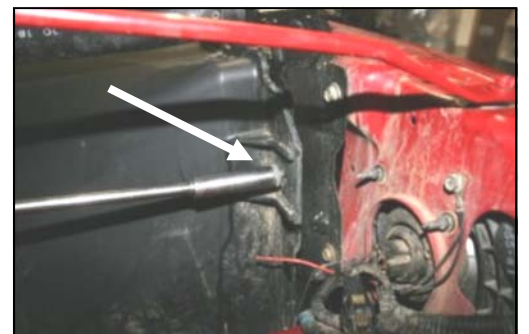
9. Remove one bolt from the passenger side radiator fan shroud and save it for step #15.
