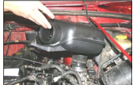
6. Remove the resonator from the vehicle.
