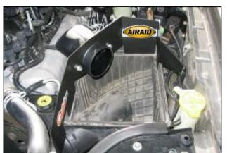
**7.** Position the Airaid Cool Air Dam in place of the factory air box and snap into place.
