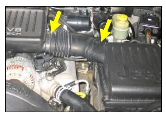
**1.** Disconnect the negative battery cable, and then loosen both of the hose clamps to factory tube connecting factory air filter assembly to factory air box silencer.
