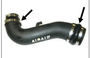
**8.** Slide the urethane hump hose and hose reducer onto the Modular Intake Tube. Use the two #60 hose clamps on the hump hose and a #56 & #52 hose clamp on the big & small ends of the reducer.
