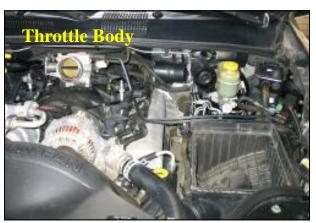
**5.** Remove the factory air box silencer coupler from the throttle body.
