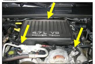
**4.** Loosen the hose clamp on the throttle body & both 10mm bolts securing factory air box silencer to intake manifold. Remove the factory air box silencer from engine compartment.
