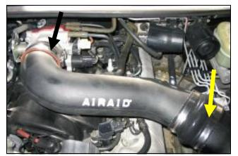
**9.** Position the Modular Intake Tube assembly to connect the reducer to the throttle body and the hump hose to the Airaid Cool Air Dam. (Note: leave the hose clamps loose until final assembly)
