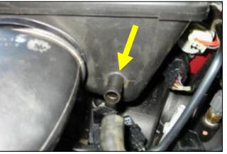
**3.** Disconnect the breather hose from the factory air box silencer.
