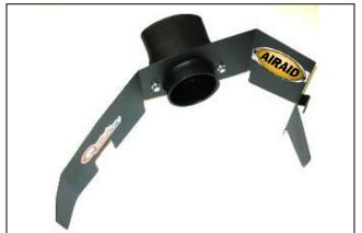
**6.** Using the two ¼-20 bolts and washers provided, fasten the black plastic filter adapter to the Airaid Cool Air Dam. Apply the Airaid Foil Decal onto the Panel as shown.
