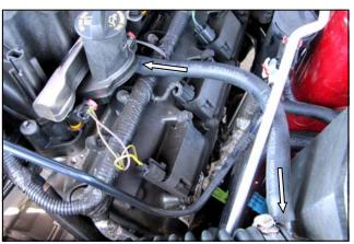
**14.** On V8 motors, replace the factory crankcase breather line with the 13" Breather Hose (#5) and connect it to the Airaid Intake Tube. Disregard the 90 deg. Elbow (#7) it will not be used.
