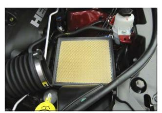
**4.** Remove the upper half of the airbox and the factory air filter.
