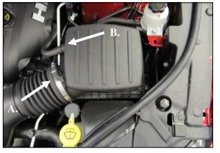
**2. A)** Loosen the hose clamp on the airbox side of the factory intake tube. **B)** Disconnect the crankcase breather line from the airbox lid.
