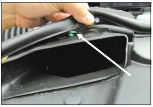
**5.** Carefully separate the hood seal from the cleat on the airbox inlet. Pull gently from side to side to avoid tearing the seal.
