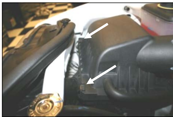
2. Unlatch the two clips on the factory air cleaner box lid.
