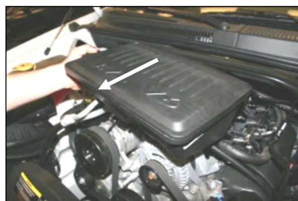
8. Remove the factory intake resonator box from the throttle body by pulling the box towards the radiator and then lifting up.
