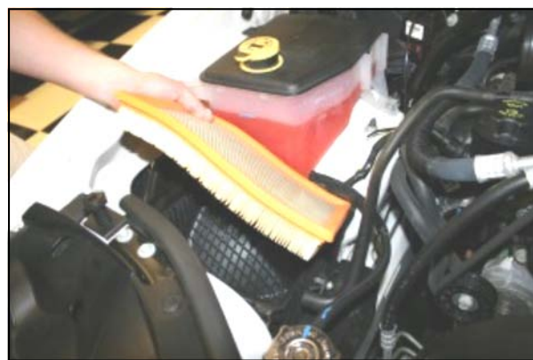
5. Remove the factory air filter.
