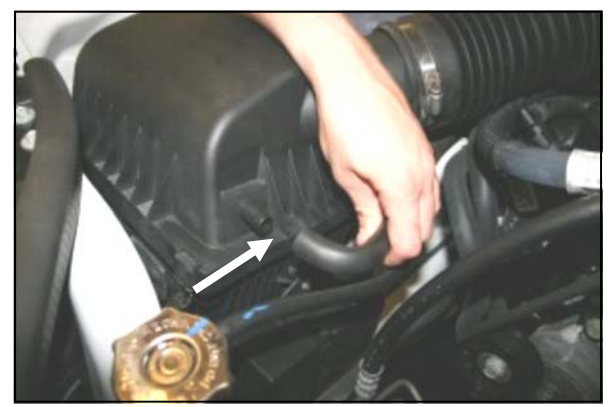
3. Disconnect the factory breather tube from the air cleaner box lid.
