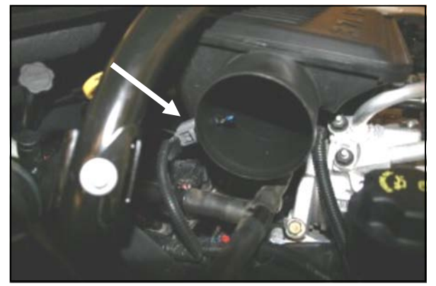
6. Disconnect the intake air temperature sensor wiring harness, by squeezing the tab on the side, and sliding the connector off.
