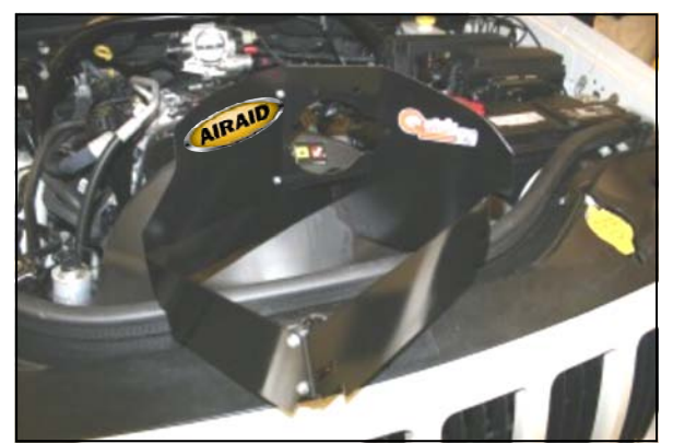
9. Assemble the Quick Fit panels as shown, using five 6-32 screws (#16), #6 washers (#17), and keps nuts (#18). Apply the Airaid Foil Decal onto the Panel as shown.
