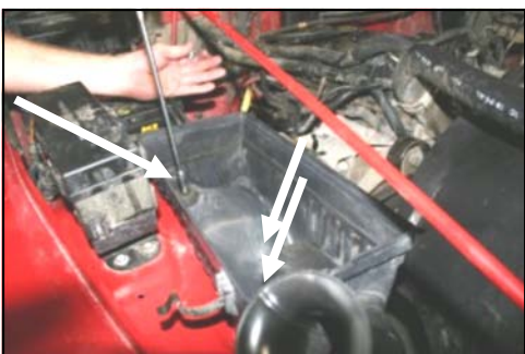
7. Remove three bolts from inside the lower air cleaner box and remove it from the vehicle.
