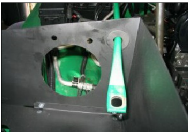
8. Position Airaid Cool Air Dam in place by inserting factory radiator support rod through grommet as shown.
