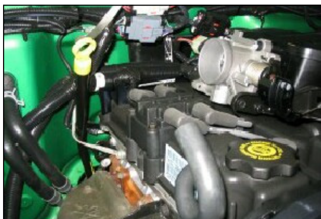
4. Remove air filter assembly from engine compartment. Retain rubber throttle body coupler for later use.
