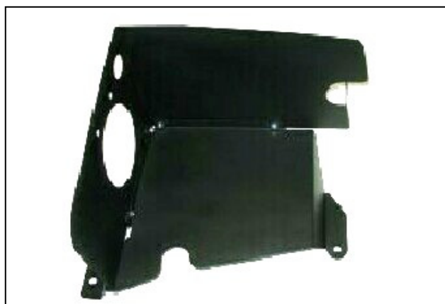
7. Using the supplied hardware, assemble the two Airaid panels as shown.
