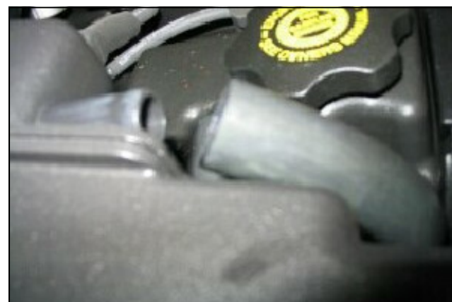
3. Disconnect the breather hose from the factory air box silencer. (Note: Retain hose for later use.)
