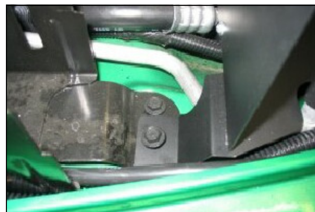
9. Reinstall original bolt through Airaid Cool Air Dam and factory fuse block bracket. Replace fuse block on bracket.
