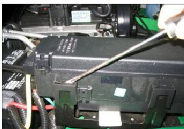
5. Using a flat blade screwdriver, unclip the fuse box from the bracket and set aside. Using 10mm socket, remove bolt from bracket. (Note: Retain bolt for later use.)
